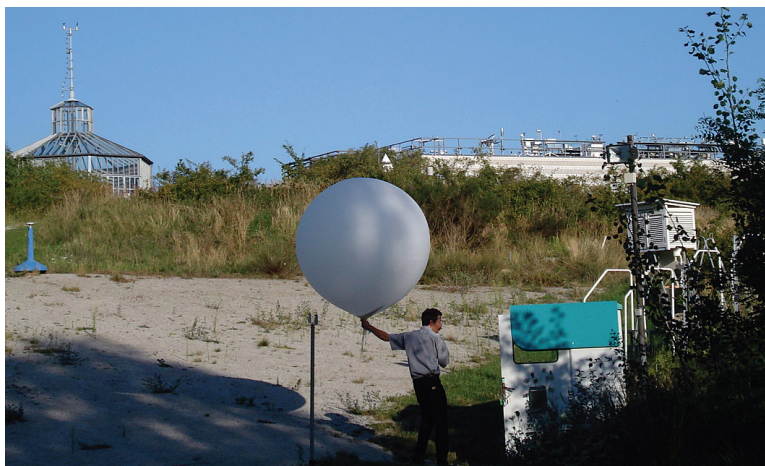
FIG. 2. The Deutscher Wetterdienst’s Meteorologisches Observatorium Lindenberg, designated as GRUAN Lead Center and the first GRUAN network station, has all the GRUAN observational capabilities depicted in Fig. 1. Here Michael Schröter prepares to launch a radiosonde and verifies that the ground station is receiving data from the sonde. A Stevenson shelter (behind bushes at lower right) houses reference surface instruments for comparison. On the roof of the radiation building (in background on right) are Baseline Surface Radiation Network instruments (pyranometer, pyrhelio meter, pyrgometer, and all-sky camera) and a microwave radiometer (far right). A GSNN antenna is to the left of the radiation building. The historic winch house (in background on left) was used in the nineteenth and twentieth centuries for meteorological profile observations with tethered aerological kites; the observatory holds the world record for achieving a kite altitude of 9,750 m on 1 Aug 1919.
